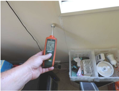
this crack is likely due to bad placement of sheet joints.
