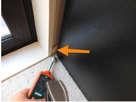
there is evidence of a leak by this door it is reading dry.
