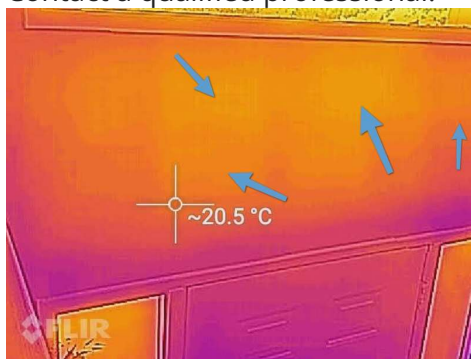
Missing Insulation above main door.
