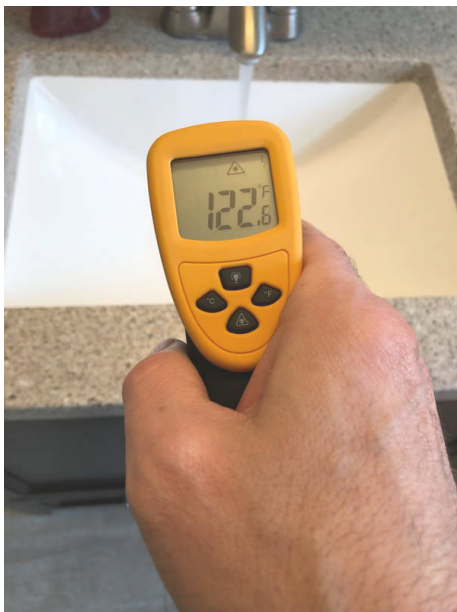
Hot water registered
