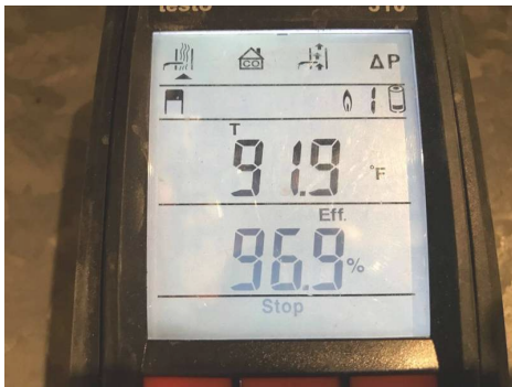
Efficiency reading. The furnace was operating at 96.9% efficiency.
