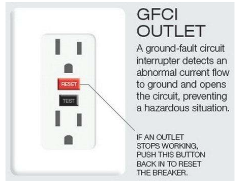
GFCI Reset Diagram
