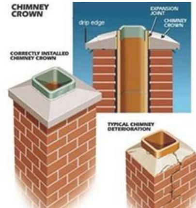
Chimney Crown Diagram
