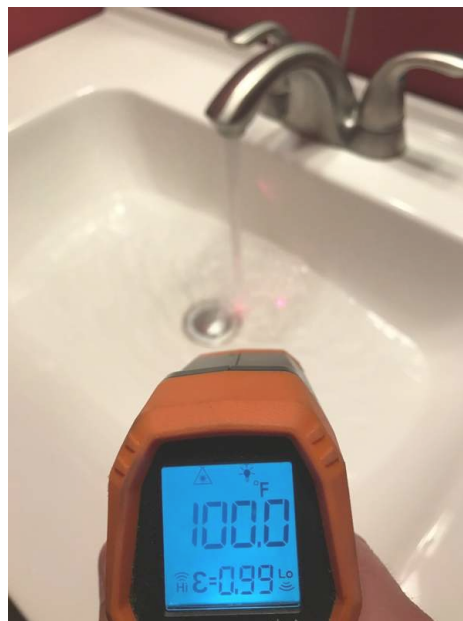
Heated Water Measured at 100 Degrees
