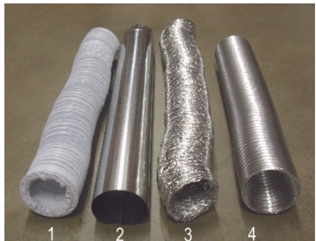
#2 or #4 best ducts for dryers
