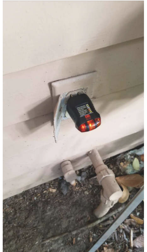
Front reverse polarity
