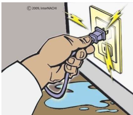
GFCI's offer shock protection in wet locations
