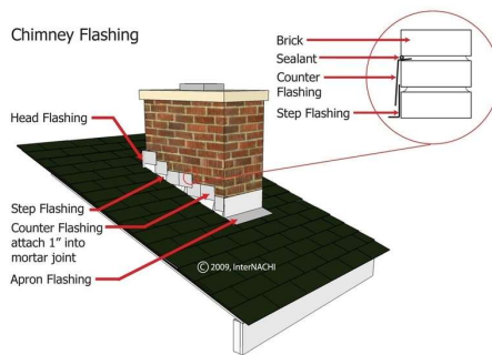
Proper Chimney Flashing Example
