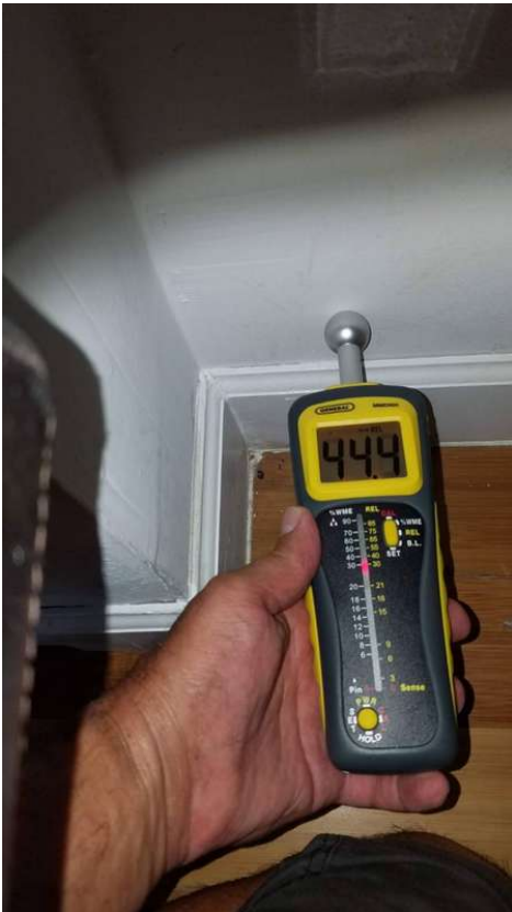
Moisture reading of 44% - should be below 10%.
