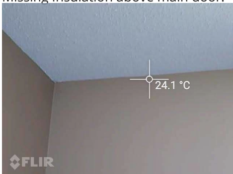
Missing Insulation above main door.
