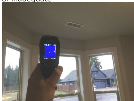
Back left bedroom - Thermal image measured cold temperatures indicating ceiling insulation is missing or inadequate
